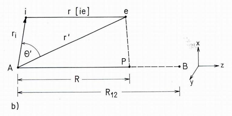
Figure 1. (a) Relative coordinates of the oxygen nucleus, introduced as a cation A, one of its electrons i and the proton P; (b) The cation A, one of its electrons i, the proton P and its electron e. R is a distance separating the nucleus A from P,  $R_{12}$  is a distance separating the nucleus of the cation A from the nucleus of the cation B.
