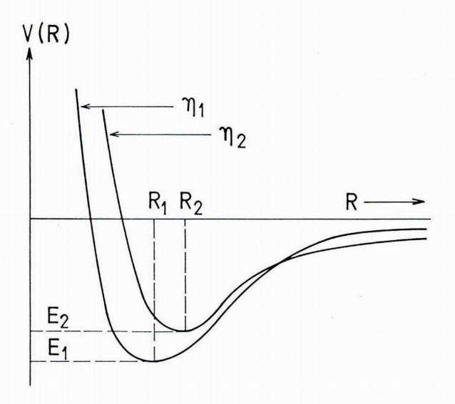
Figure 2. Potential energy of a proton V(R) as generated by the oxygen cluster (nucleus +8 electrons) plotted qualitatively as a function of the A-P separation distance R, for two different values of the contraction parameter  $\eta$ , where  $\eta_1 > \eta_2$ . Notice also that  $|E_1| > |E_2|$ , while  $R_1 < R_2$ .
